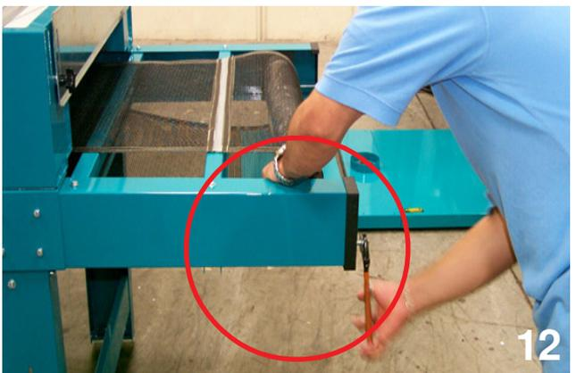
Start the Dryer with the Belt running about 35% and as the Belt heats up make very SMALL adjustments to keep the Belt tracking in one position by turning the adjustment screw Clock wise to bring the roller end OUT or Counter Clock wise to push the Roller end in.
