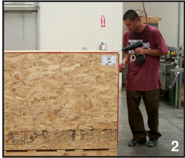
The POWERHOUSE Dryers (2608, 3011, 4013, 5217) ship in one wooden Crate (Photo 1). Uncrate using a power screwdriver (Photo 2).
