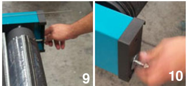
Pull out the Joining Pin that is stored in one of the Belt ends.
