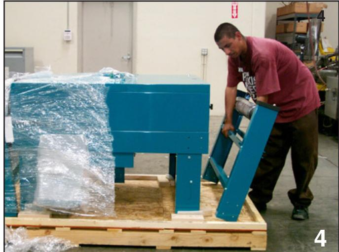
Remove the shrink wrap ( Photo 3). Then remove the Belt Extensions. DO NOT REMOVE THE SHRINK WRAP on the Belt Extensions these hold the Belt Rollers in place (Photo 4).
