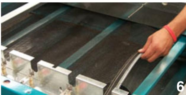
Pull the Belt out of the Heat Chamber OVER the TOP Belt Extension Braces (Photo 7).
