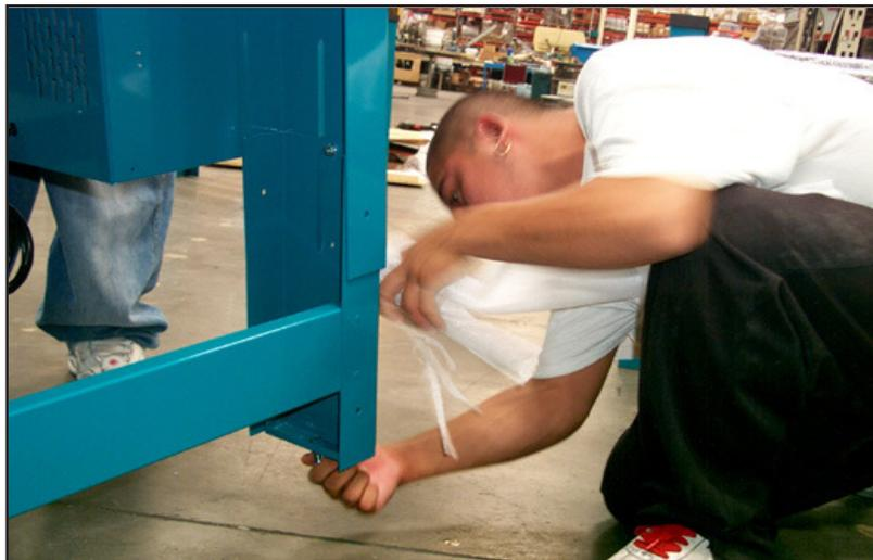
**DO NOT** try to raise the level of the Dryer with the Stabilizing Bolts and **DO NOT** use casters on the Dryer legs as this will cause damage to the metal structure. If the Dryer is not level lift the Dryer leg that will make it level before you attempt to adjust the Stabilizing Bolt.
