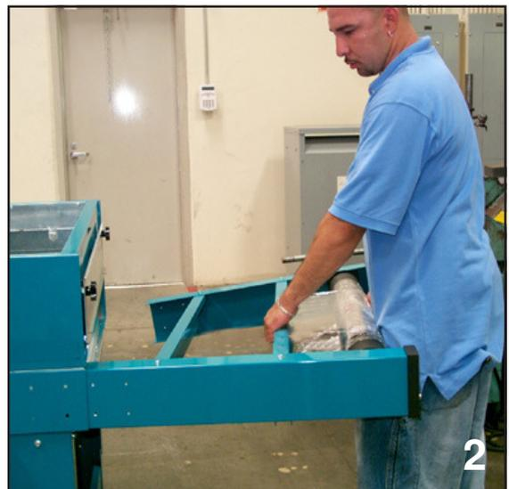
Insert the Arm Assemblies into the body of the Dryer making sure that the support arms have the smooth side facing up (Photo 2).
